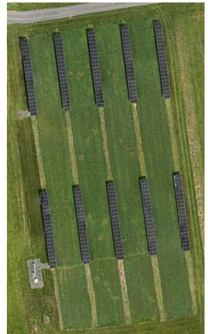
Figure 1: Rutgers University Snyder Farm with a single-axis tracker array installed with an intentional -7° azimuth adjustment and 32 feet row spacing.
