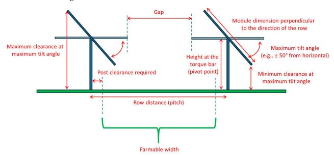
Note: Supports for some single-axis tracker arrays consist of post configurations with a wider ground-level footprint causing a possibly smaller farmable width. For taller equipment, the farmable width may end up being only as big as the gap (with additional clearance needed on both sides). Also, some array brands have driveshaft components that connect between rows. This may also impede full length access along the rows depending on the specific geometry.
