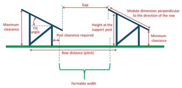
Note: Some fixed-tilt arrays use a single support post with a cross-brace for each row, which might allow a larger farmable width, depending on having equipment fit under the array on either high or low side.
